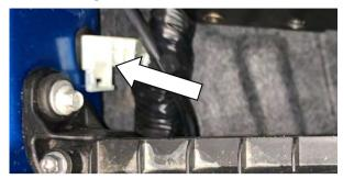
3. Remove fasteners (rear half only) for RHS inner guard and lower.
