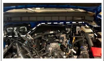
36. Pickup power from the stability bar module fuse (10A) located in the engine bay fuse box. Fuse reference #158 in owners manual.
