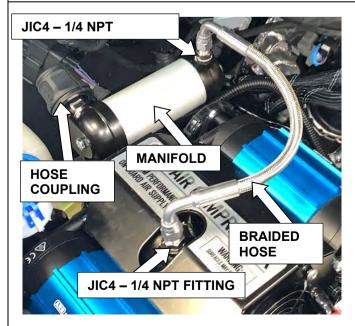
29. Using the fittings provided in the kit 171503, fit 1 x JIC4 - 1/4 NPT fitting to the inboard manifold port (as shown in the image to the left).
