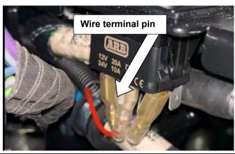
38. Connect spade connectors from wire to switch pin 2.
