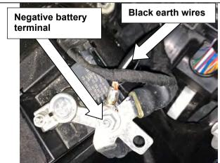
40. Connect up the 2 black earth wires from the compressor wiring harness to the negative battery terminal.
