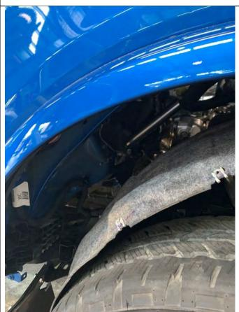
4. Fit the rear support bracket (4655173) using the factory OE M8 flange bolt. Leave loose at this stage.
