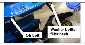
23. Temporarily remove the washer bottle filler neck by removing the bolts retaining it to the vehicle body.
