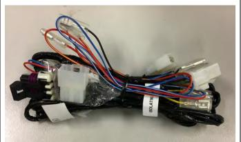
33. Using the wiring harness 180415, measure and cut 400mm of wire (purple/black) connected to the purple plug.
