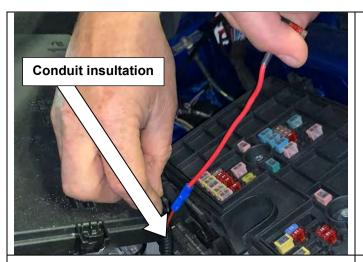
37. Run wiring around the rear section of engine bay to the compressor switch.
