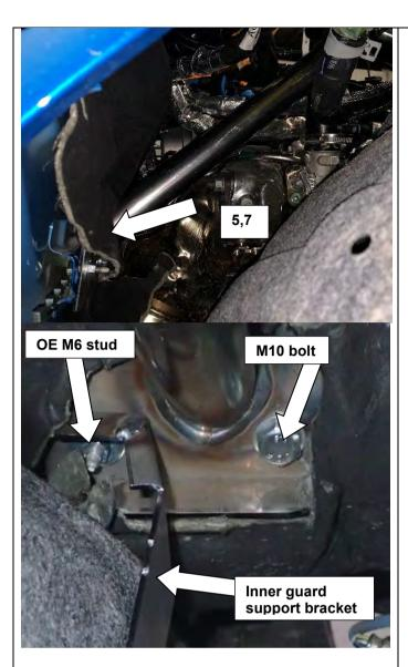
Feed support tube weldment to the firewall and locate onto the M6 stud. Once on, place the inner guard support bracket over the same OE factory stud, and fasten OE M6 nut.
